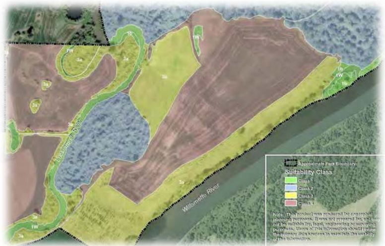
During park planning efforts, OPRD’s natural resource staff evaluate the vegetation, wildlife, and forest resources of the subject parks. This information is synthesized into a composite map (example above) that highlights what areas are best suited and what areas unsuitable for future park development.
