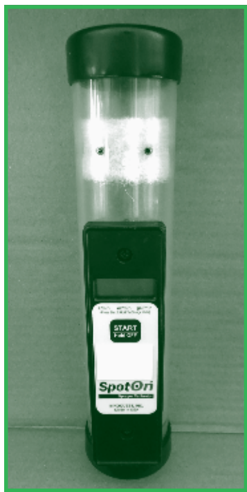
Figure 11.2 A device to measure nozzle flow.
