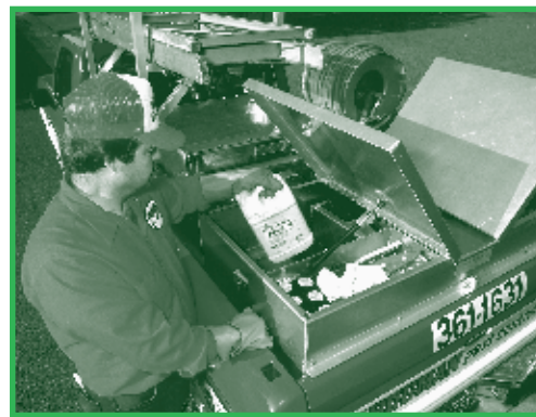
Cargo boxes allow for secure transport of pesticides and help prevent theft and vandalism.
