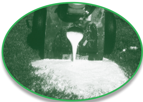
Physical incompatibility results in an unsprayable mixture, in this case, excessive foaming.
