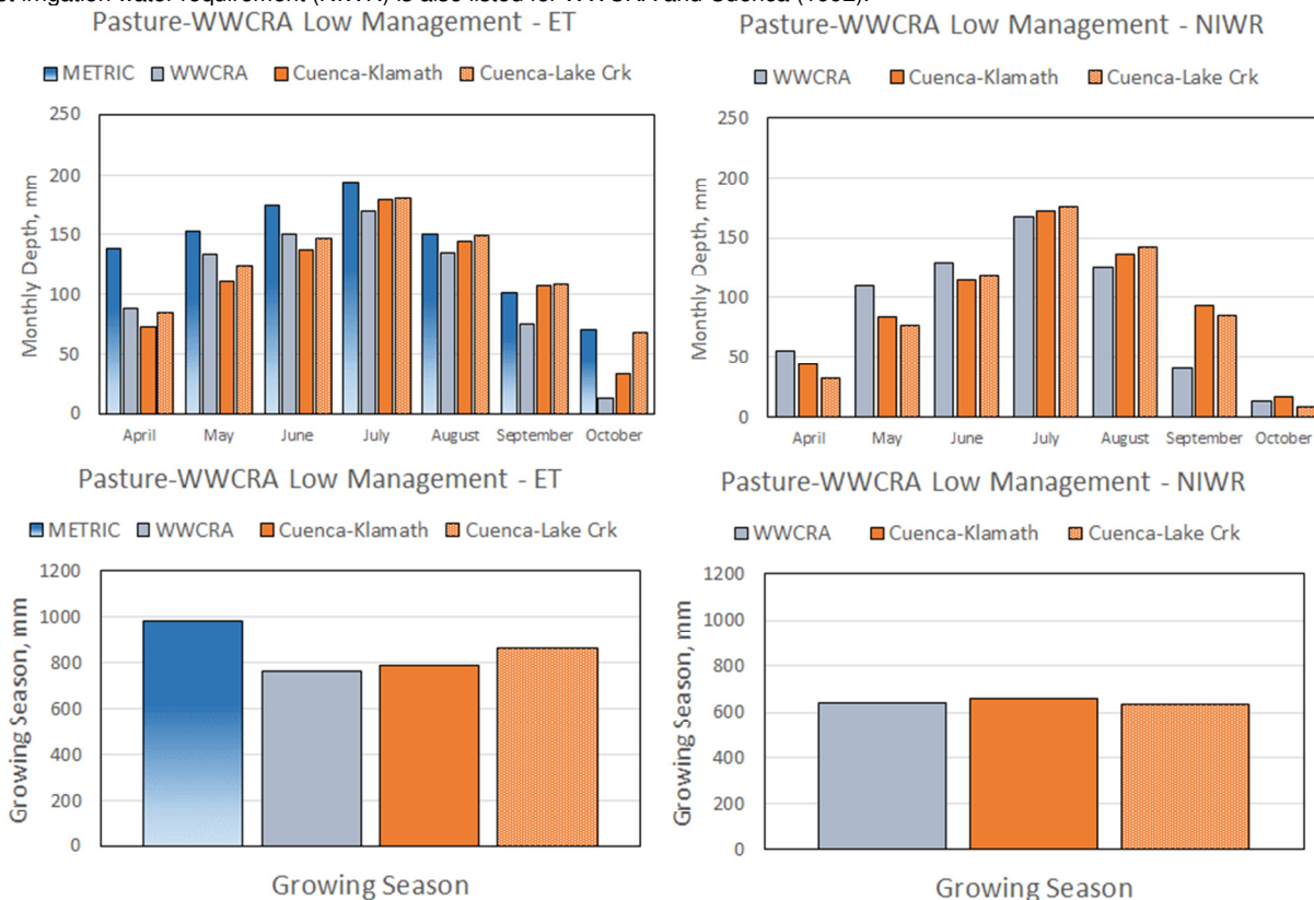
Figure 11. Comparison of Monthly ET for Grass Pasture (upper left), Monthly NIWR (upper right) and Growing Season Totals for year 2013 (METRIC and WWCRA for the HUC 18010204 Klamath SE subbasin) and for Historical Cuenca (1992) Estimates for Klamath and Lake Creek / Little Butte Creek Units of Cuenca
