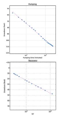
Variations in these curves can be used in determining the type of aquifer (confined, unconfined) and any flow boundaries<sup>3</sup>. Transmissivity is calculated using the pumping rate and drawdown over one log-cycle. A poorquality test may look something like the example below, where pumping rate was not held constant.
