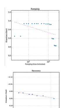
The water levels during the pumping phase show a sharp dip at the beginning of the test followed by a variable rate of drawdown.
