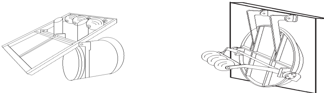
Figure 1-3. Self-regulating tide gate (SRT, top), which is default open. Top-hinge tide gate with mitigator device (bottom), which is open for a portion of the incoming tide.
