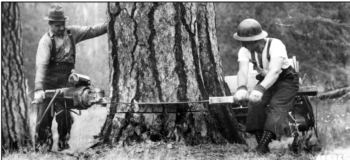
"Felling a tree using an electric power saw," from Malheur National Forest, USFS photo #426966 (Gerald Williams Photo Collection, OSU, retrieved at oregondigital.org)
