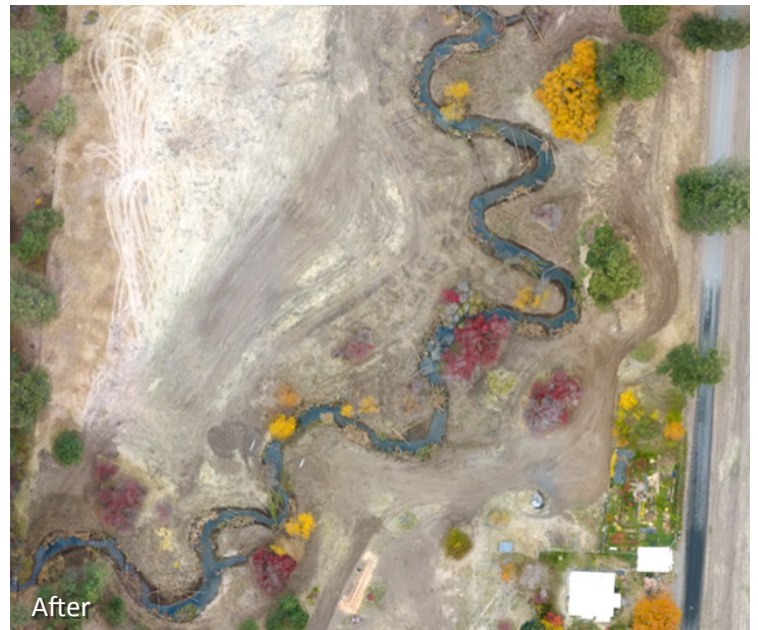
Before restoration at Dry Creek, the stream banks were incised and the floodplain was less than one acre. The Union Soil and Water Conservation District worked with a private landowner to restore the creek's sinuosity and floodplain, doubling it in size. The stream habitat was further enhanced by placing 280 large trees and 600 pieces of wood and planting more than 5,000 native plants.
