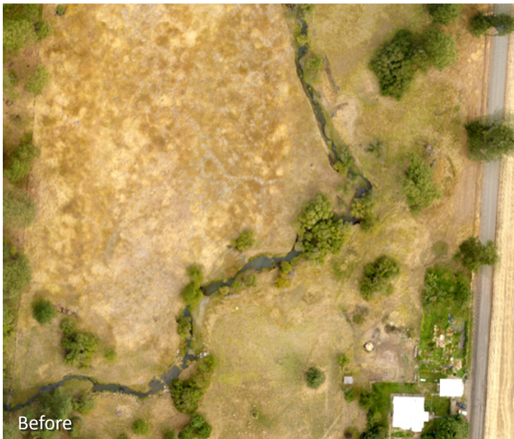
Before restoration at Dry Creek, the stream banks were incised and the floodplain was less than one acre. The Union Soil and Water Conservation District worked with a private landowner to restore the creek's sinuosity and floodplain, doubling it in size. The stream habitat was further enhanced by placing 280 large trees and 600 pieces of wood and planting more than 5,000 native plants.
