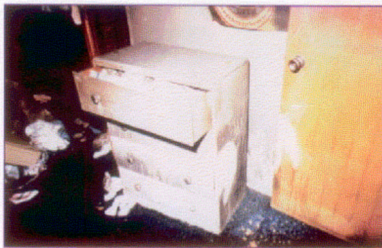
A closeup of the first victim's location. Notice the smoke and heat demarcation in the bedroom area of the home. (CS9-6)
