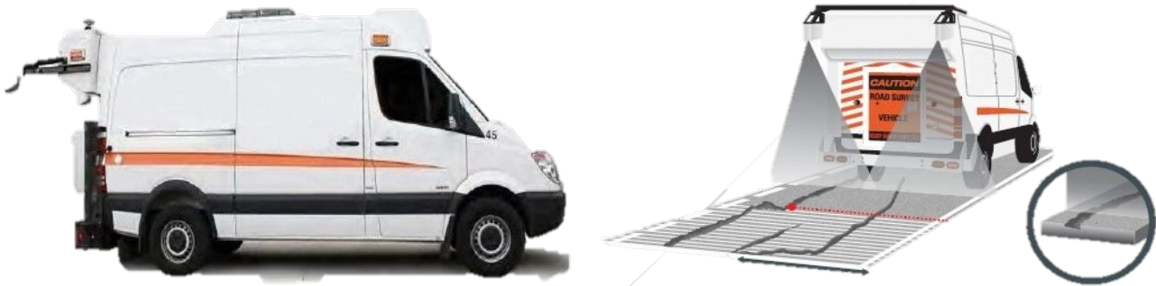
2-6 Pavement Data Collection Vehicle used for Automated Distress Survey
