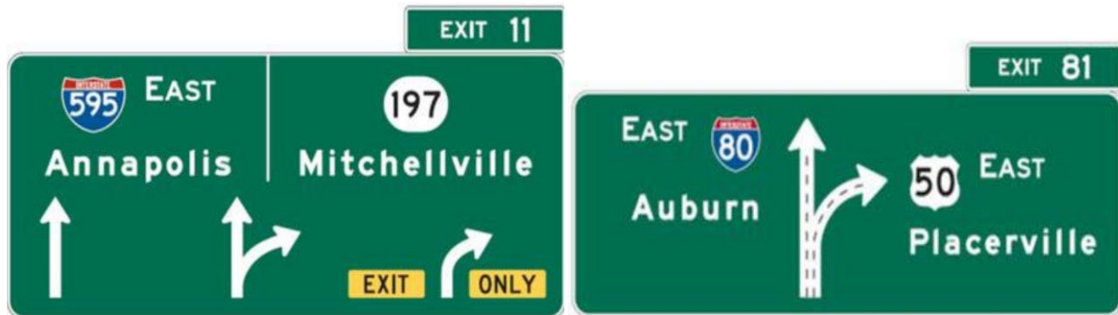
Figure 2.5: A comparison of arrow-per-lane guidance sign (left) and standard diagrammatic guidance sign (right) (MDOT, 2015)
