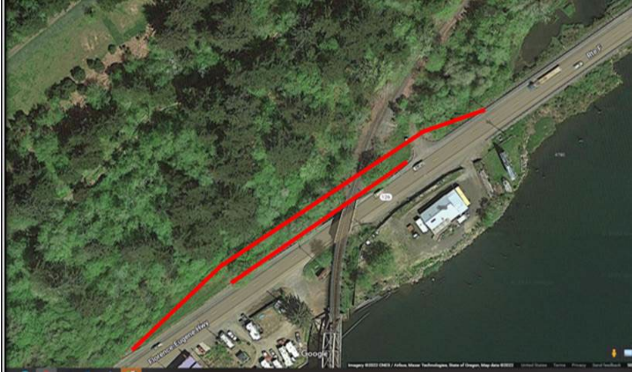
Image 5 – One possible solution would be to construct a short bypass around the area vulnerable to flooding. This would be a one-lane, bi-directional roadway, controlled by signals on both ends. It would only be open during flood events. It would be closed (with movable barricades) during other times.
