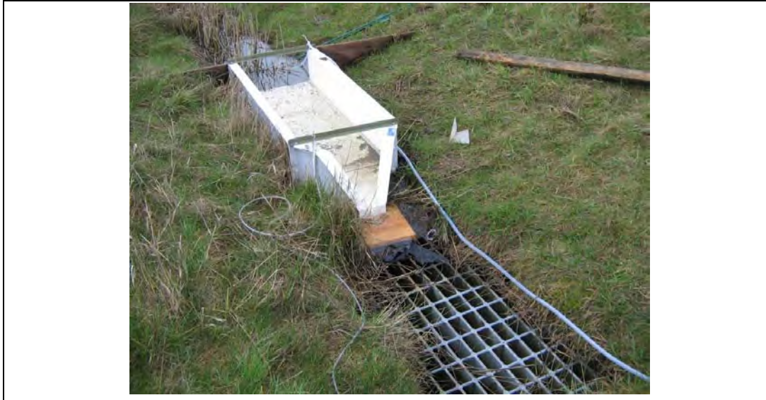
Figure 5-1. Flume to collect stormwater runoff from Interstate 205 in Washington State, Herrera Environmental Consultants.
