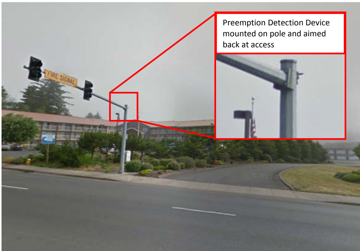
Figure 17-10 | Preemption Detection Device – Placement Example
