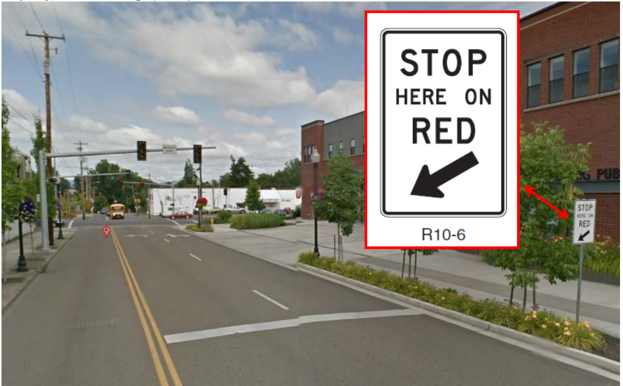
Figure 17-8 | Stop Here on Red Sign (R10-6)
