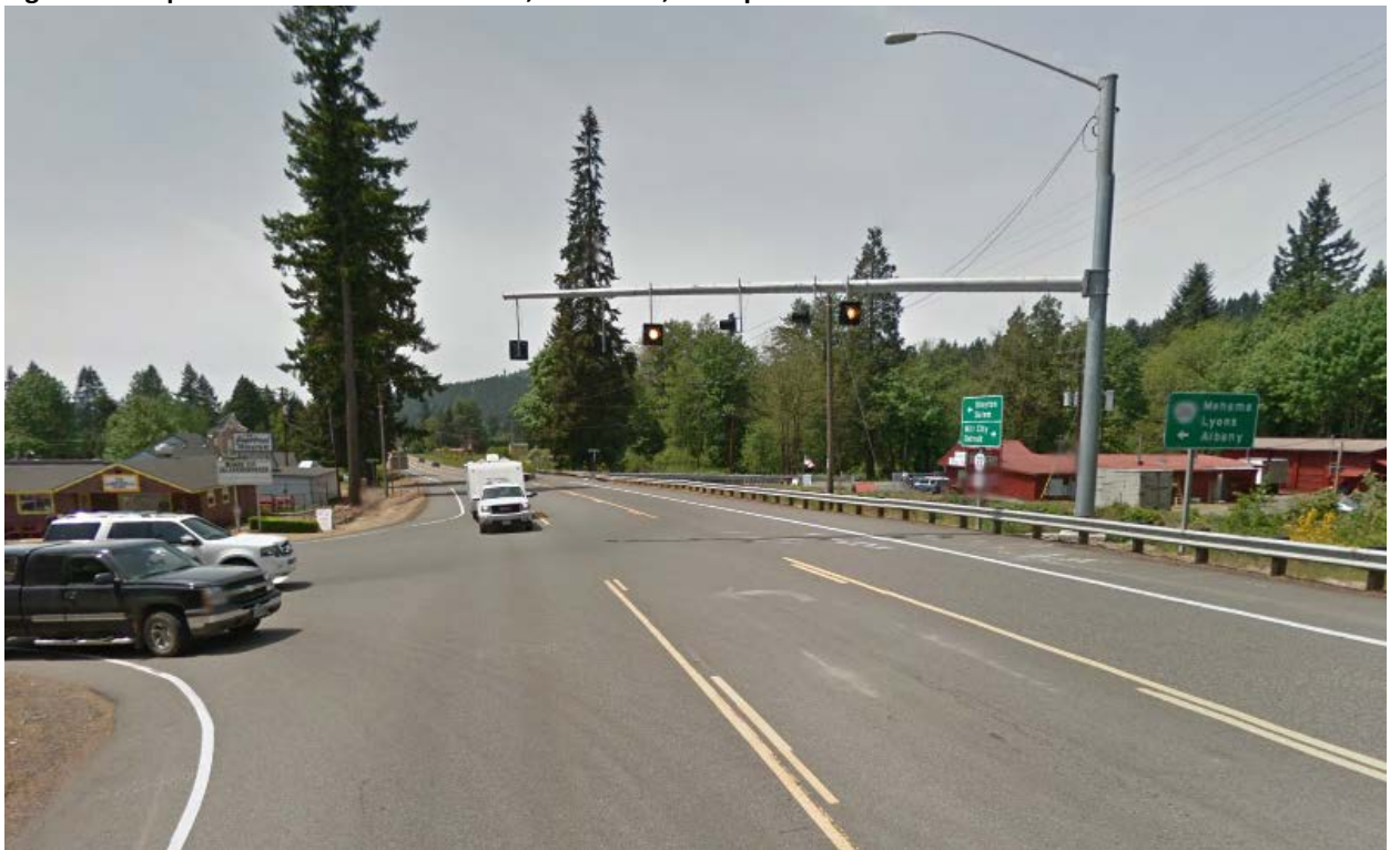
Figure 12-16 | Intersection Control Beacon, Mast Arm, Example 2
