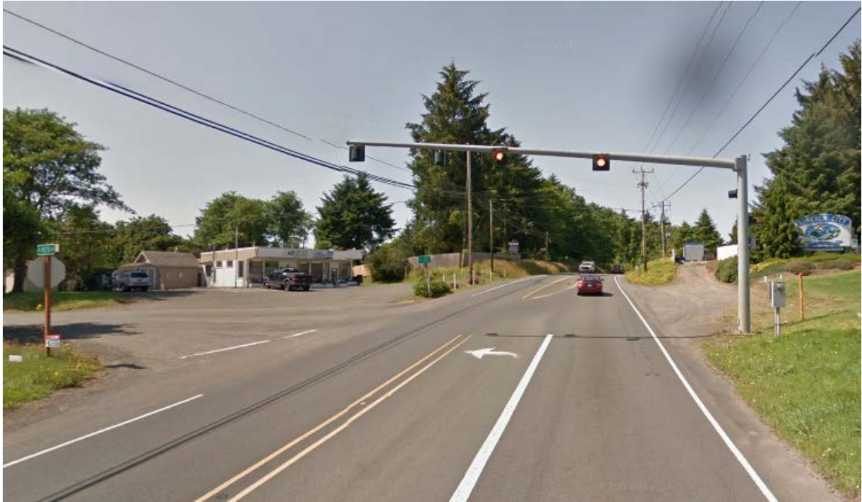
Figure 12-15 | Intersection Control Beacon, Mast Arm Example 1
