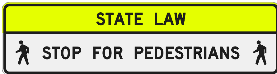
Figure 189: Overhead Pedestrian Crossing Sign (R1-9a)
