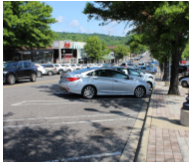
Typical Head-in Diagonal Parking Reduced Visibility to Oncoming Vehicles and Bicyclists
