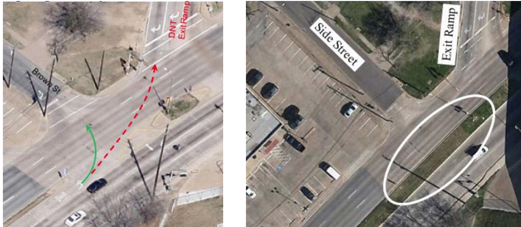
Figure 3-33: Before (left Image) and after (right Image) Narrowing a Median Opening on the Crossroad, (Zhou and Pour Rouholamin 2014c; Zhou 2014d)
