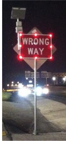
Figure 3-39: RRFB Wrong-Way Sign (left), LED Wrong-Way Sign (right), (Finley et al. 2014; Lin et al. 2016a)
