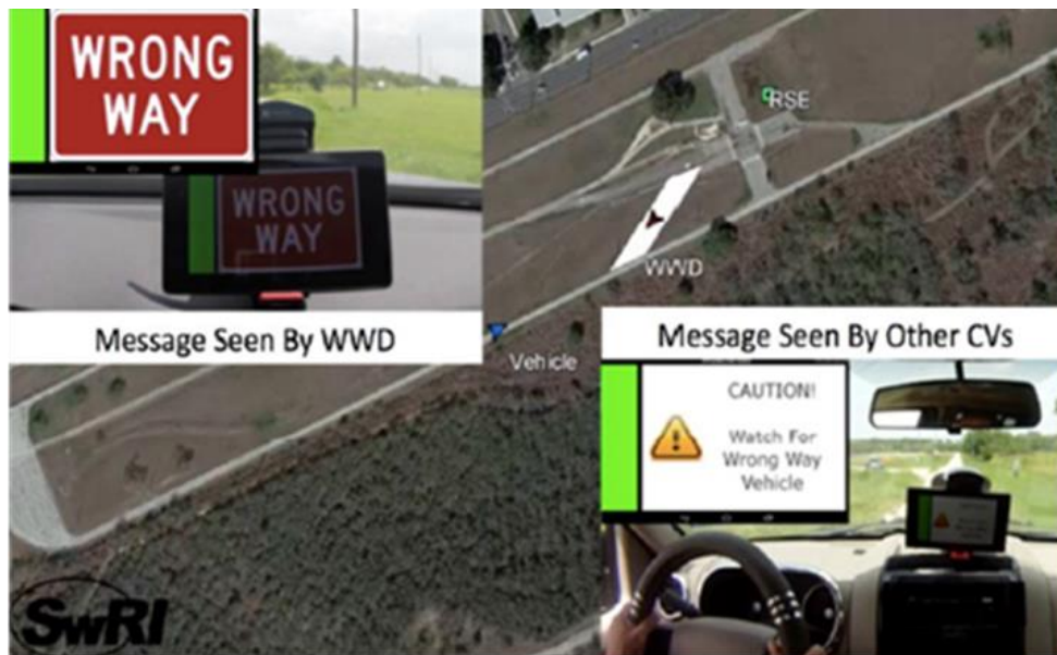
Figure 3-44: Connected Vehicle WWD Messages Sent By RSE, (Kockelman et al. 2016)
