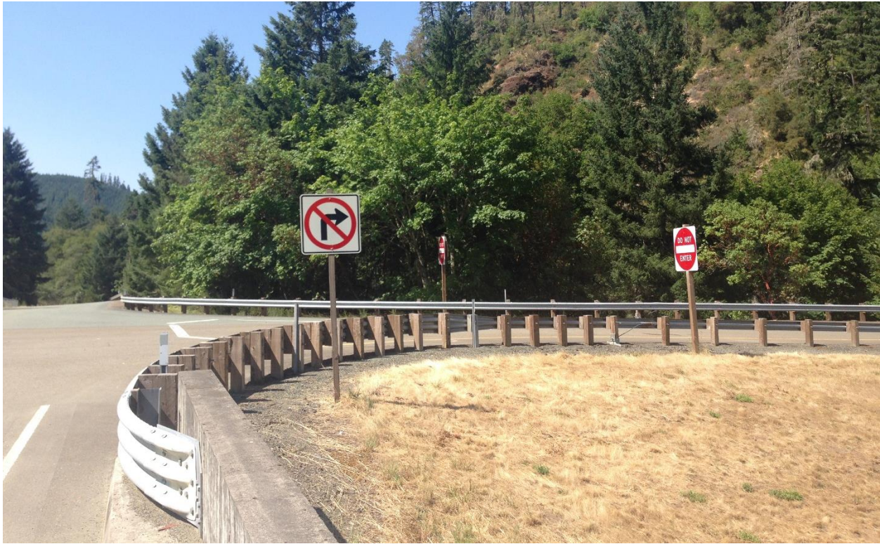
Figure 5-6 Turn Movement Prohibition Sign
