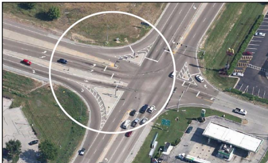
Figure 3-35: Use of Median to Divide the Same Direction of Traffic, (Zhou and Pour Rouholamin 2014a)
