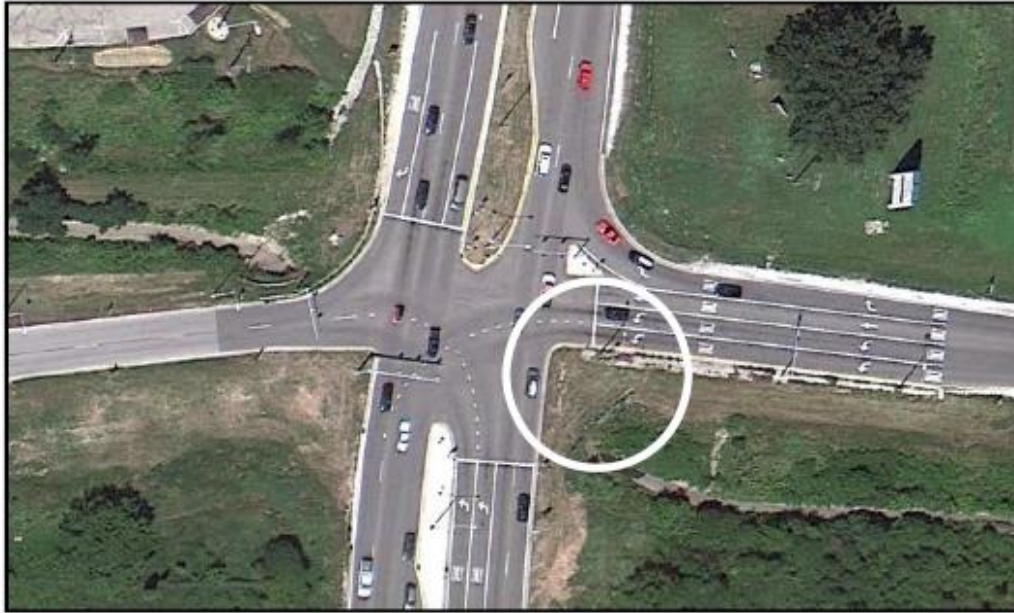
Figure 3-30: Example Angular Corner at the Left Edge of the Exit Ramp, (Zhou and Pour Rouholamin 2014a)
