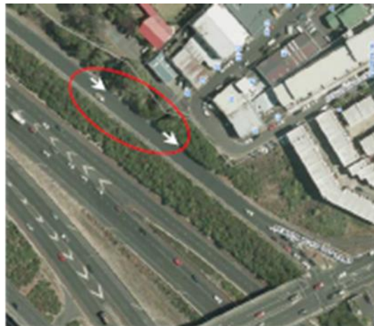
Figure 3-11: Supplemental Direction Arrows Indicating Wright-Way of Travel, (Baisyet et al. 2015)
