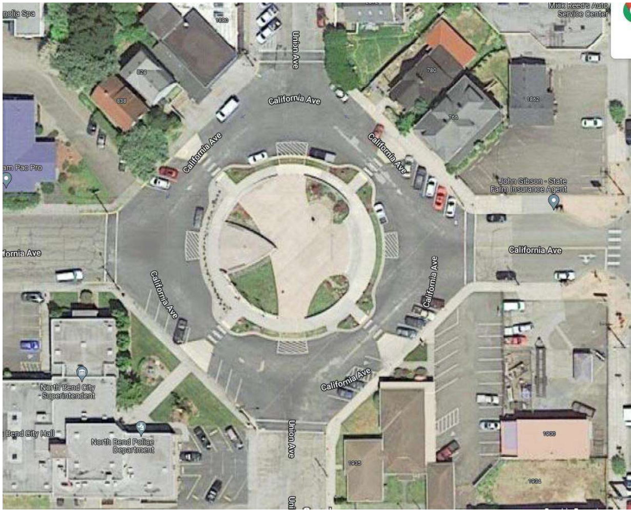
Traffic Circle with Pedestrian Access to Center Island in North Bend, OR.
