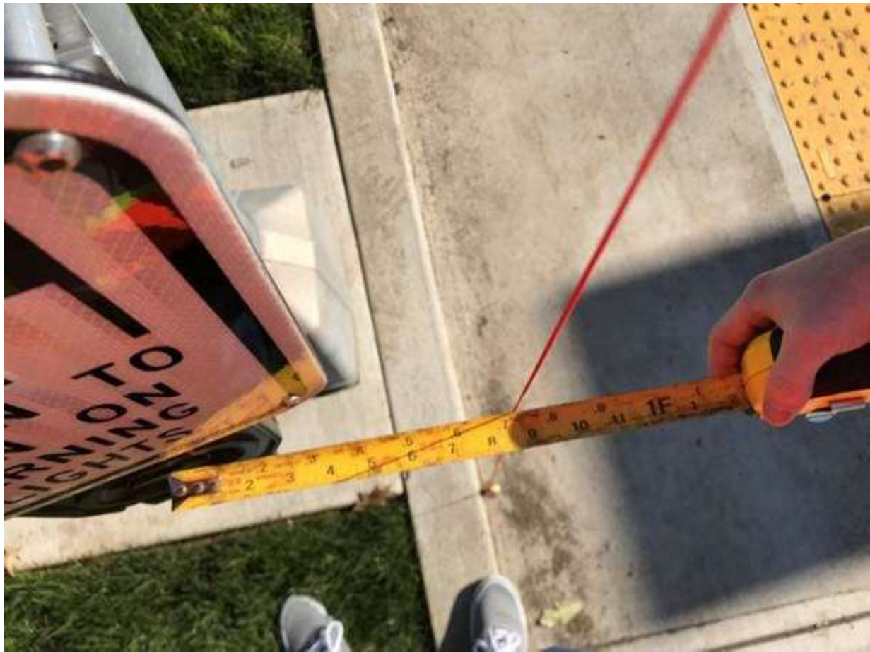
How the Reach Range Distance is Measured with Plumb Bob and Tape Measure
