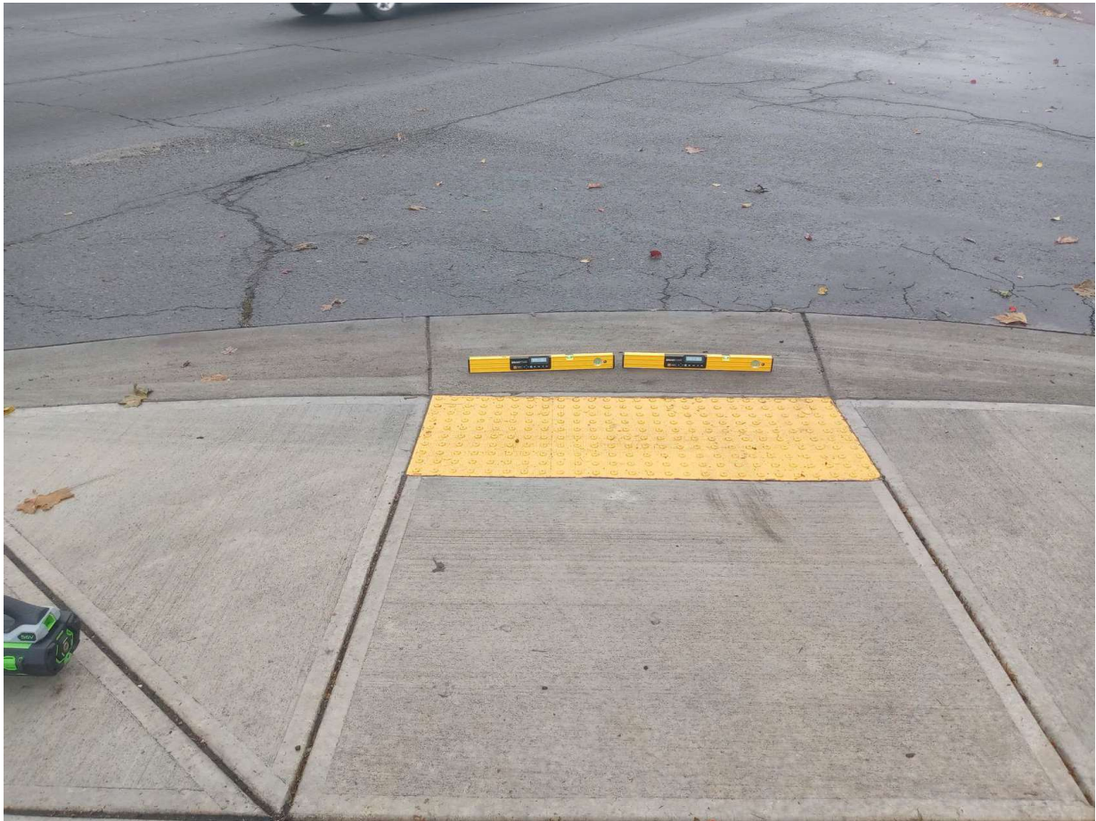
How to Measure Gutter Flow Slope
