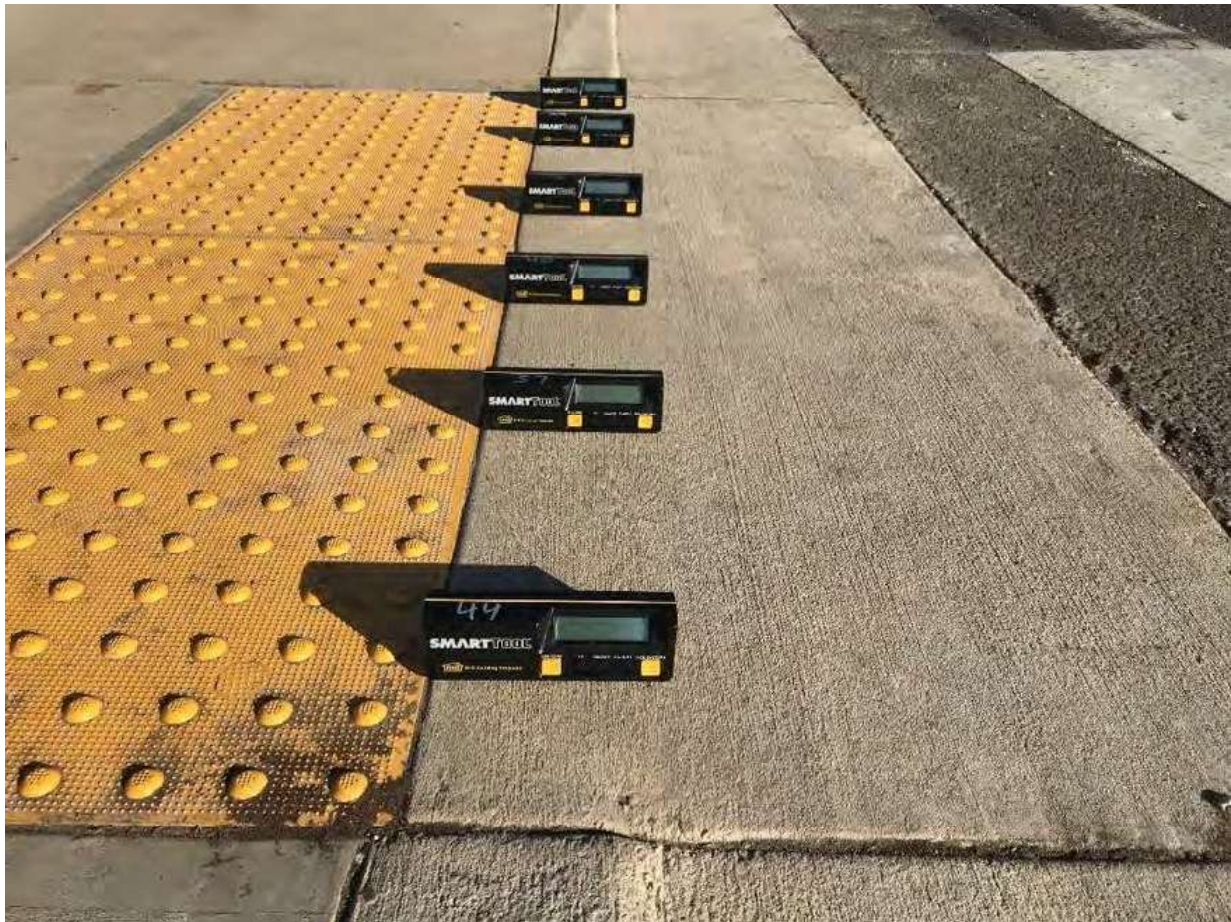
Placement of 6-inch Smart Level on a Curb Running Slope
