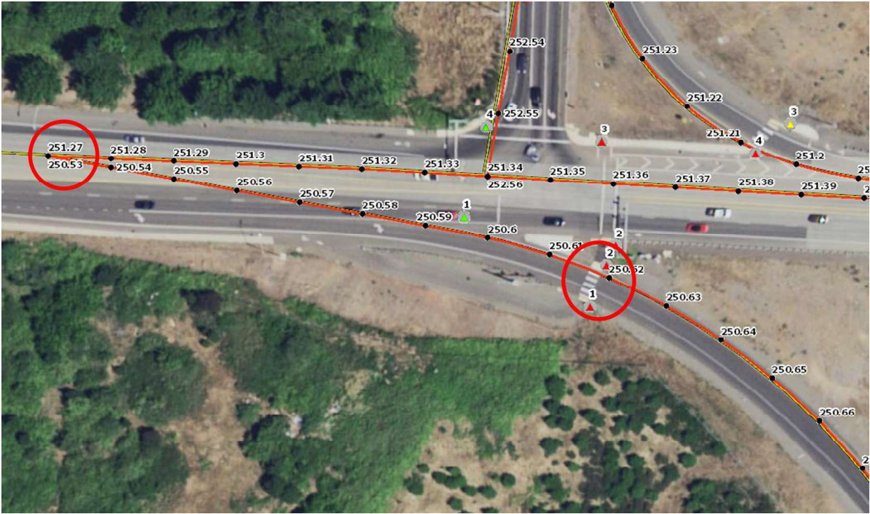
Example of a Gore Mile Point designation for On-Ramp Curb Ramps. Use MP 251.27 from Mainline Highway on Overpass
