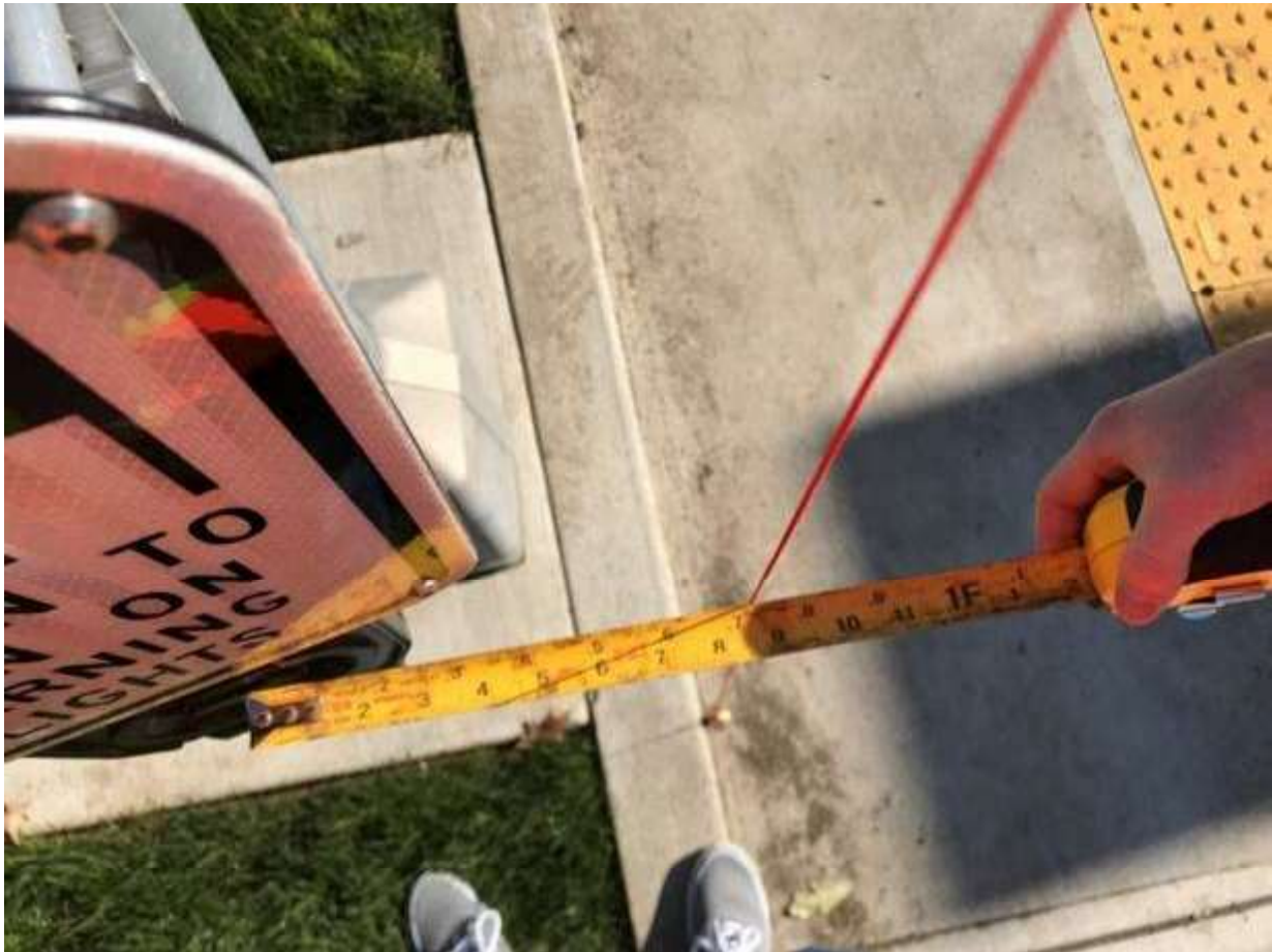
The picture above shows how the reach range distance is measured with plumb bob and tape measure for the push button inspection form.
