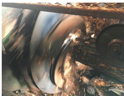
The narrow opening of a mill's small-diameter "ring debarker" is just one part that limits log size (Source: Eric Simmons, US Forest Service).
