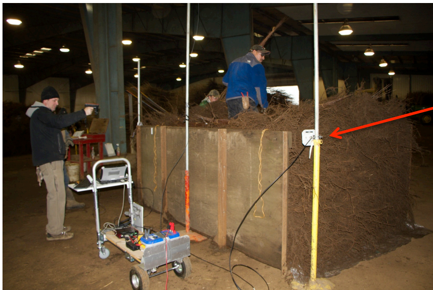
Figure 4: A full pallet showing probable bundle signal interference with the 4 foot mounted antenna.
