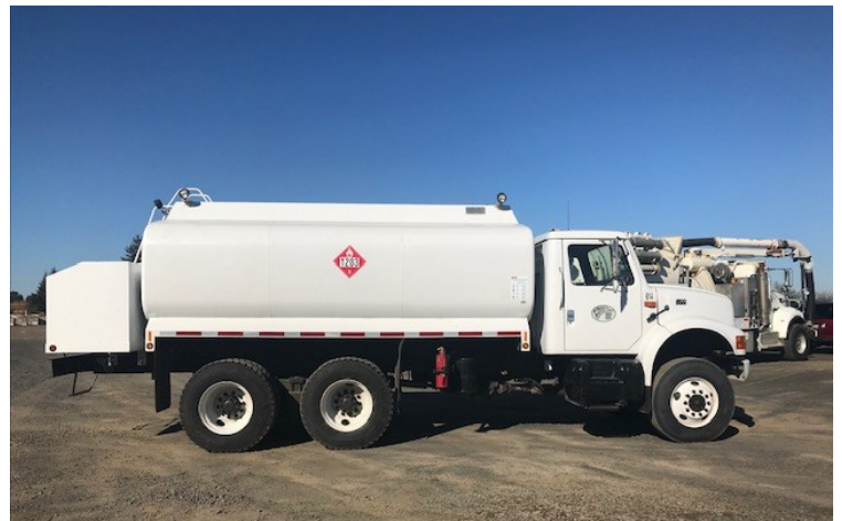
McMinnville's fuel truck holds up to 2,000 gallons of diesel and 250 gallons of gasoline.
