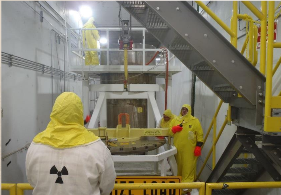
STSC and trailer in the K West Basin Annex during operations demonstrations for the contractor-led ORR
