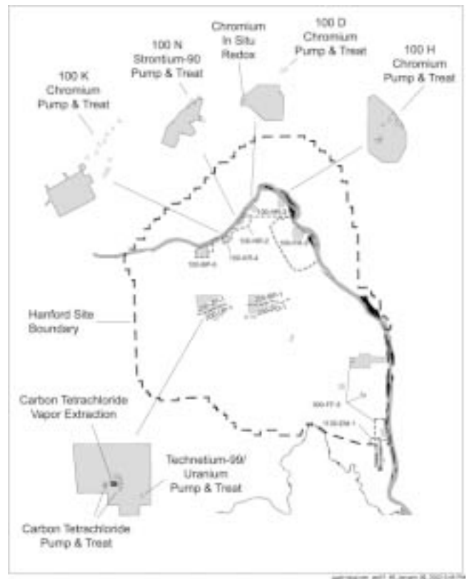
Pump and treat and other groundwater contamination containment systems at the Hanford Site
