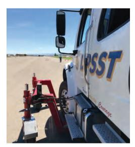
What exactly is a skidtruck? The skidtruck is a semi-truck that has been modified with a set of "training wheels" that are controlled from within the vehicle. The skidtruck system uses hydraulic rams and casters to lift the truck just enough to limit the normal traction and simulate driving on wet pavement, snow, ice, etc. With this system DPSST is able to teach drivers how to stay calm while employing techniques that keep the driver in control when navigating hazardous conditions.
