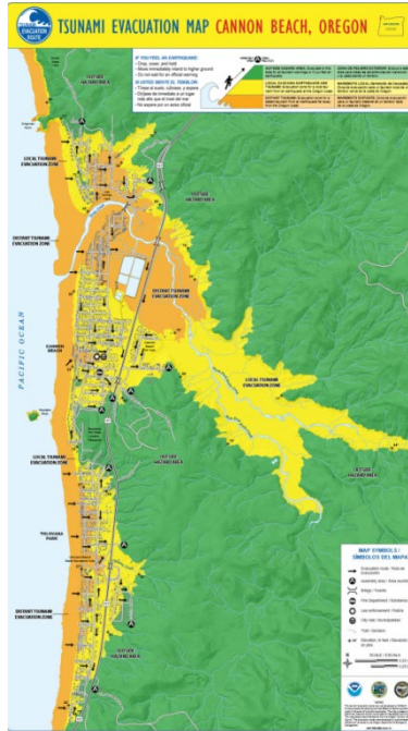
Figure 2. DOGAMI (2013) tsunami evacuation map for Cannon Beach. Inundation for a maximum-considered Cascadia subduction zone (CSZ) tsunami scenario (XXL) is shown in yellow, while the maximum-considered distant tsunami scenario is shown in orange; note the Cascadia scenario encompasses both the yellow and orange zones. High ground outside the XXL hazard area is green.
