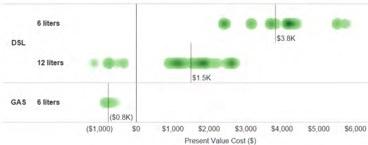
Figure 18. Present value life-cycle cost for all EMFAC vehicles in the low-cost scenario, segmented by fuel type and engine displacement (DSL = diesel, GAS = gasoline)
