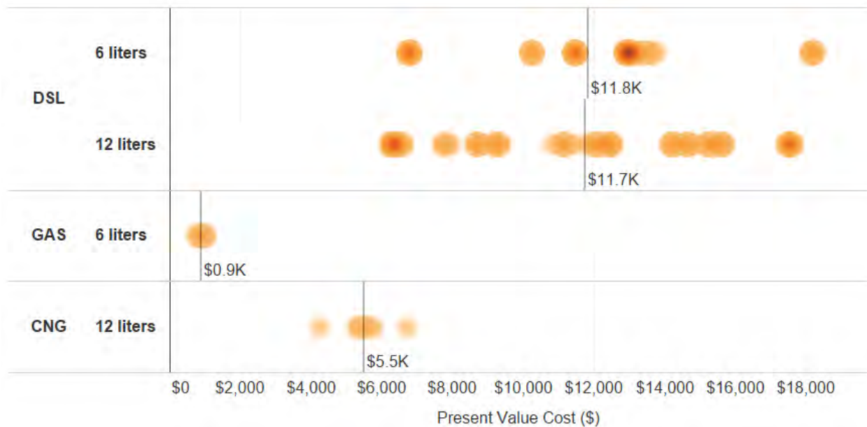
Figure 19. Present value life-cycle cost for all EMFAC vehicles in the mid-cost scenario, segmented by fuel type and engine displacement (DSL = diesel, GAS = gasoline, CNG = compressed natural gas)
