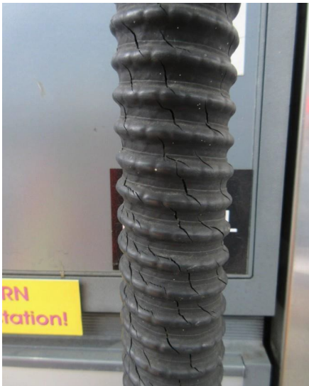
(AQGP-23) Balance System hose tears
