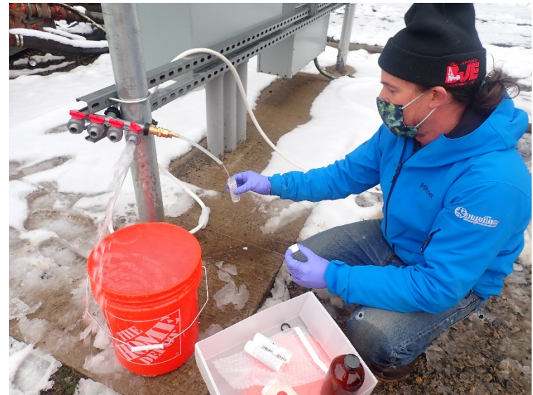
View of ground water being sampled from a barbed fitting on the sample manifold.
