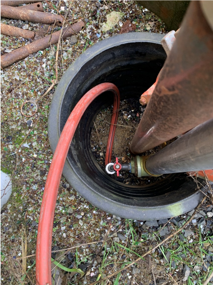
A garden spigot connected to the well head inside the well monument provided access for sampling. Note: the pictured hose was not utilized for sampling collection.
