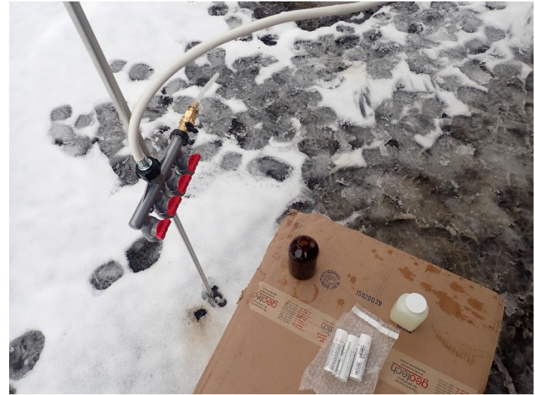
View of sampling manifold and hose connected to the spigot on the wellhead during sampling.
