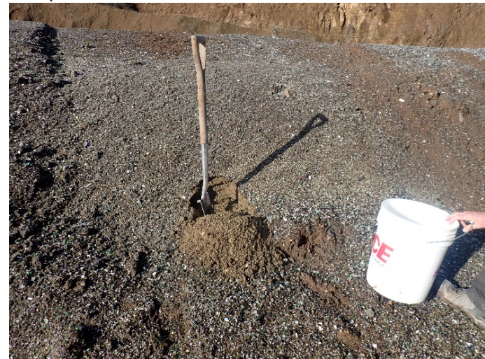
40 increments of cullet were collected from DU02 using a decontaminated stainless-steel trowel and stainless-steel hand auger.
