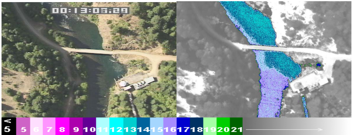
Frame: nfb0164 - N. Umpqua River at the Slide Creek Power Plant at river mile 70.32. The outflow of the power plant lowers the water temperature of the N. Umpqua River. The flow direction is from the bottom to the top of the image.
