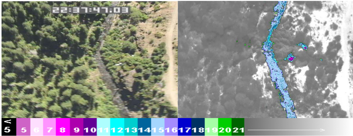
Frame: nfu0619 - Image pair showing the confluence of the N. Umpqua River (15.6°C) and Dorothy Creek (11.6°C).
