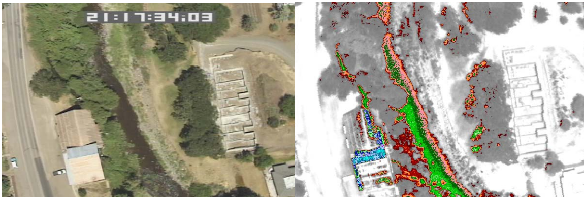
Frame: lb0582: Confluence of the Little Butte Creek (25.8°C) and canal return (24.4°C) at river mile 5.1 in the town of Eagle Point. The canal has a cooling influence on the stream, although both have temperatures over 24°C.
