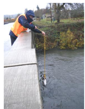
Lab staff member collecting water from a bridge monitoring site.
