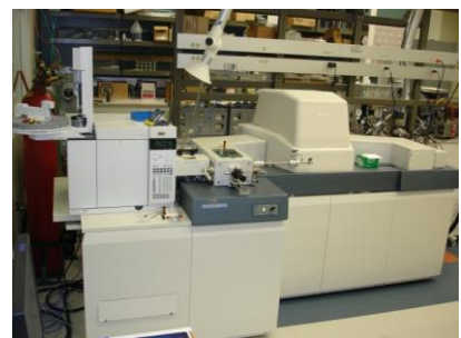
Gas chromatograph high-resolution mass spectrometer (GC-HRMS) used to analyze water samples for chemicals at sub-nanogram per liter levels.
