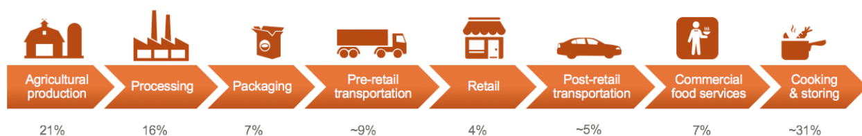
FIGURE 1. Generic life cycle of food production with the distribution of the estimated 10.8 EJ of energy used annually by the US food system based on data from the early to mid-1990s. Adapted from Heller and Keoleian, 2003. (EJ = 10 18 J).
