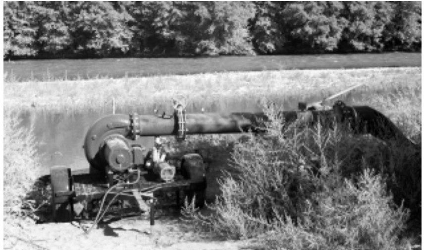
Landowners have replaced push up dams with pumps to deliver irrigation water, benefit the fishery, and conserve water. (Photo by Bob Brown/Division of State Lands)
